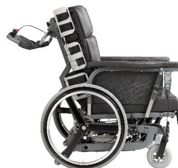
The leg rests can be dismantled without using tools.
