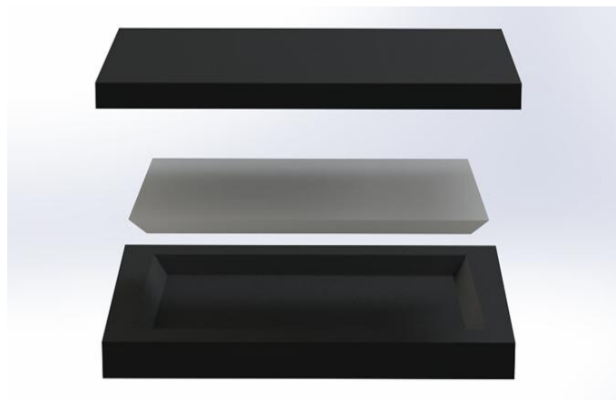
The seat cushion is made up of three diverse types of foam.
