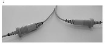
Connect the cables of the right and left motor to the two extension cables and from the control box. The right motor cable is marked on the cable clip corresponding to on the cable from
