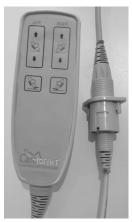
Connect the hand control to cable  $(\mbox{\sc B})$  and connect the power cable  $(\mbox{\sc 0})$  to the mains. The hand control cable is marked  $(\mbox{\sc 3})$  on the cable clip corresponding to  $(\mbox{\sc 3})$  on the control box cable.
