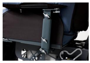
Armrest with three thumb screws on the side.
