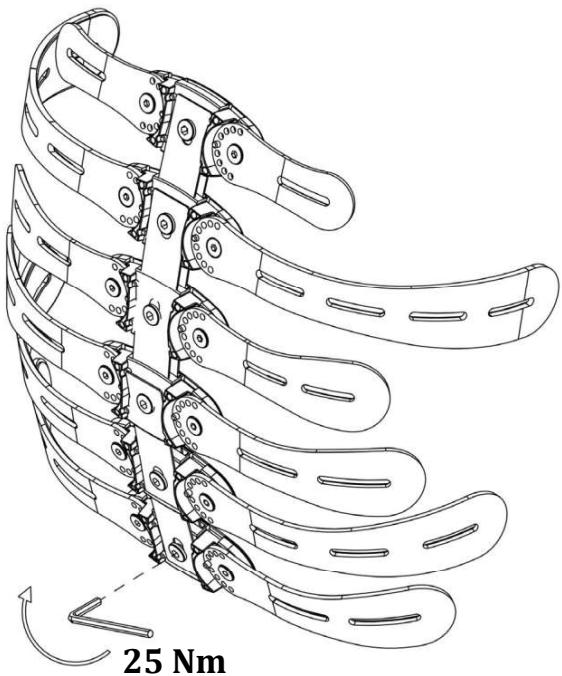
**tighten the screws to 25 Nm
