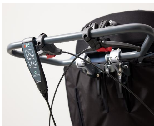
The push bar is mounted on the brackets, where the thumb screws can be found on the sides.
