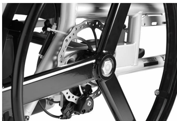
Minimaxx Wheelchair with disc brakes.
