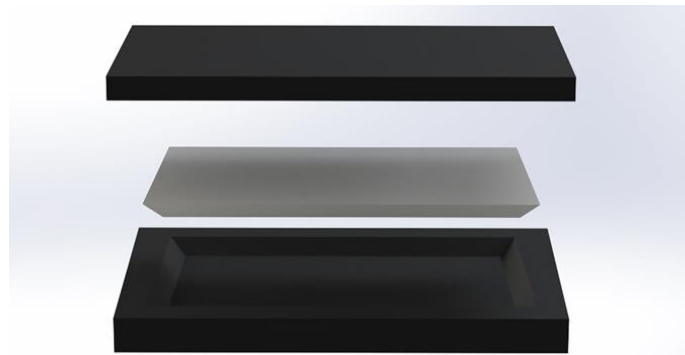
The seat cushion is made up of three different types of foam.
