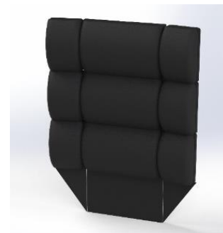
The back cushion is made up of nine modules sewn into one large cushion.
