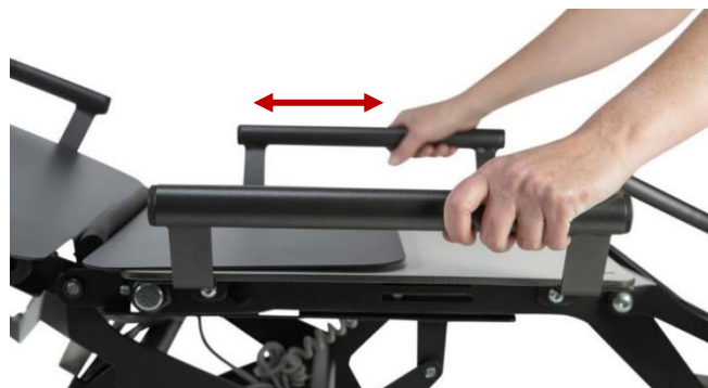
3. Grab the frame and pull it or push it to the desired position. Lock the bolts on both sides again. Pull or push the frame again until you hear a click. The frame is now locked in position.
